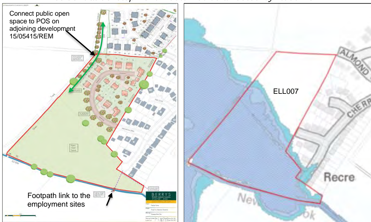
Fig 6: Proposed layout plan (left) and detailed Flood Risk Assessment (right) Residential development would not be affected by flood risk
