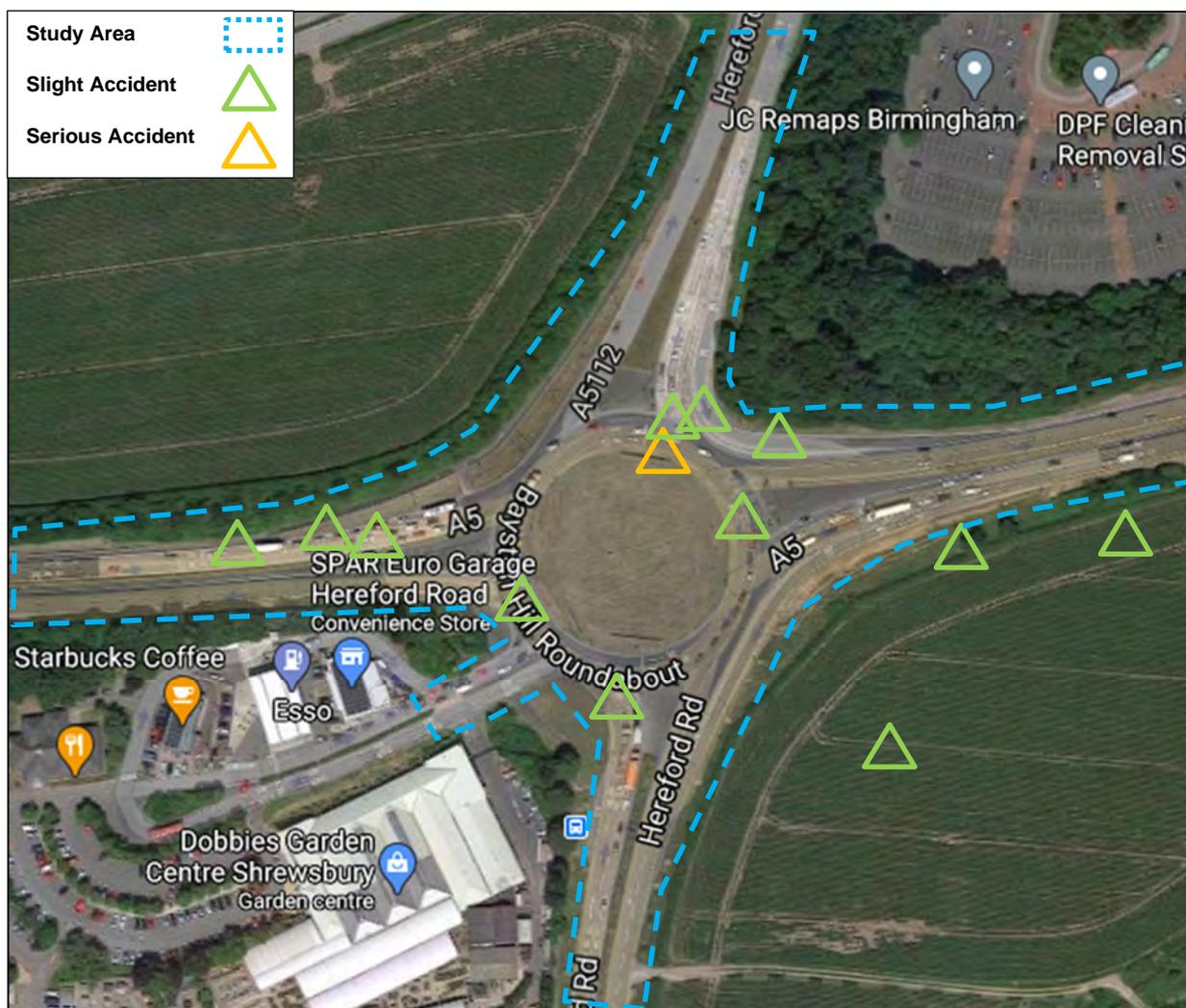
2.17 A total of thirteen accidents occurred at the Bayston Hill Roundabout over the 5-year period, twelve of which resulted in 'slight' severity injuries and one resulted in 'serious' severity injuries. Based on DMRB research presented in TD16/07, a 5-arm roundabout would be expected to experience around 3.80 accidents a year, nineteen accidents over a typical 5-year period.
