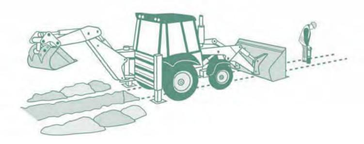
By hand, dig trial holes to locate the exact position of all cables.
