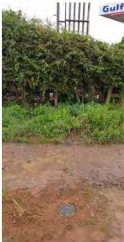
Photo 6: BH2 in relation to the PFS. Vent pipes for the USTs visible approximately 4 m from BH2
