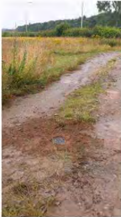
Photo 5: BH2 completed on site in the centre of the access track to the north of the PFS
