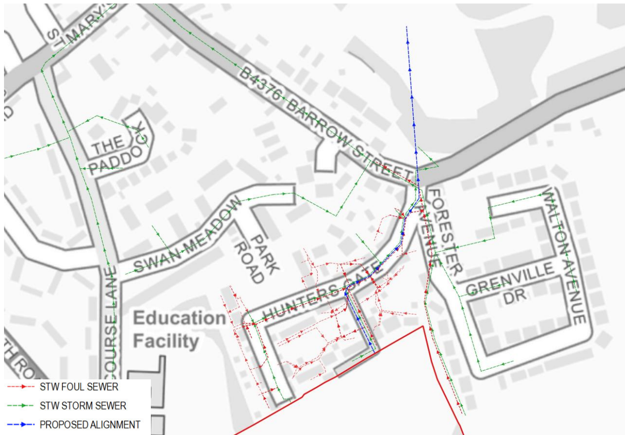
Figure 12 Proposed Culvert Alignment
