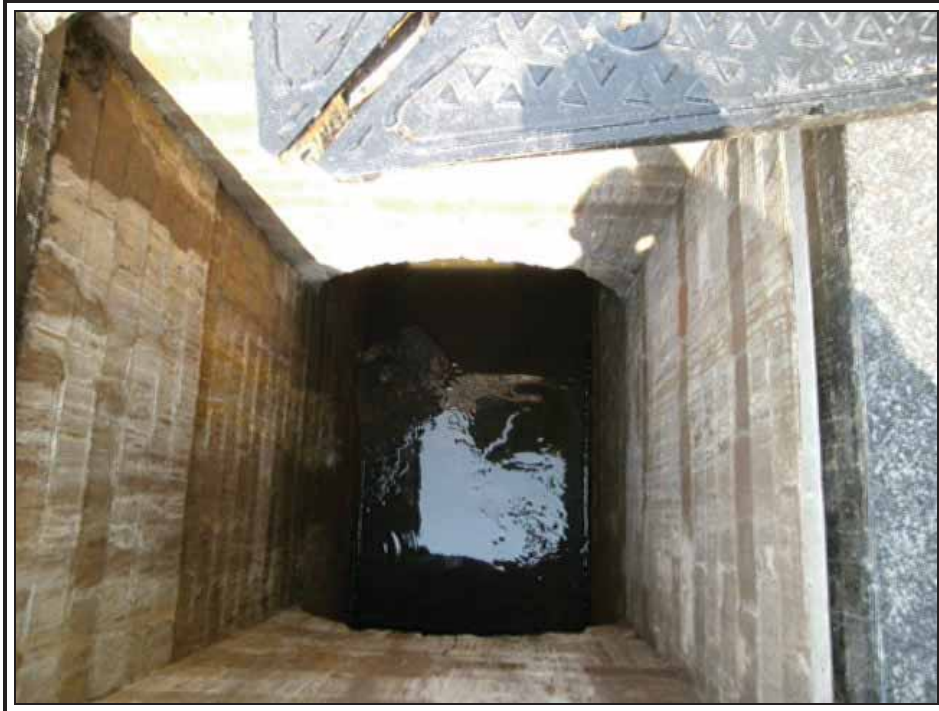
Photo 17, Tracing Dye located in manhole
