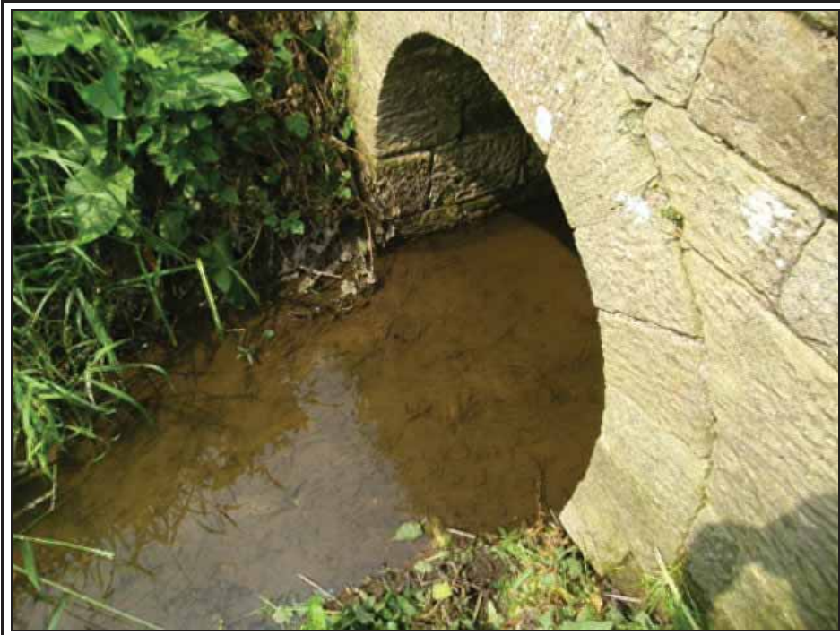
Photo 19, Tracing Dye in Outfall
